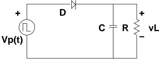
Figure 3: A rectifier powered by a variable duty-cycle pulse source.
