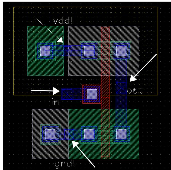
Fig. 10: Inverter Layout with Pins
