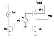
14. Calculate the output resistance of your designed amplifier.
