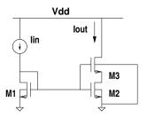
12. In the figure below,  $V_{DD} = 1.6$  V,  $I_{ref} = 50$   $\mu$ A,  $(W/L)_1 = (20\mu m/1\mu m)$  and  $(W/L)_2 = 3(W/L)_3 = (10\mu m/1\mu m)$ .
