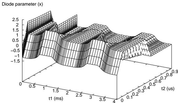
Figure 5: Bidimensional plot of the diode parameter ( $x$ )
