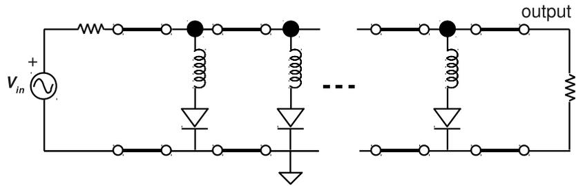
Figure 4: Nonlinear transmission line (soliton line)
