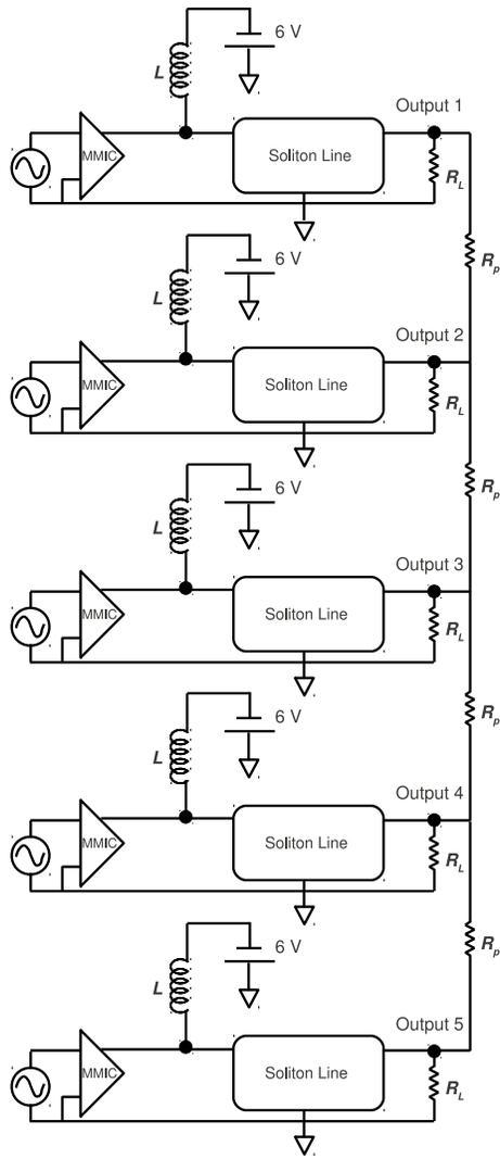
Figure 5: Multi MMIC-Soliton-line schematic
