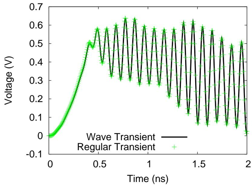
Figure 10: Output voltage of the X-Band MMIC array spacial power combiner
