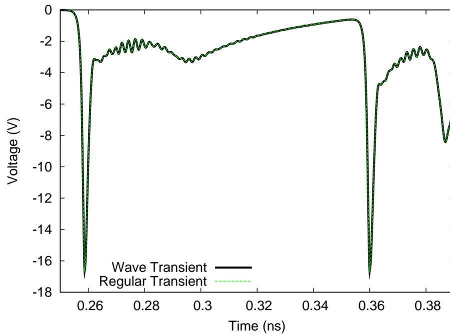
Figure 8: Output voltage of Soliton Line
