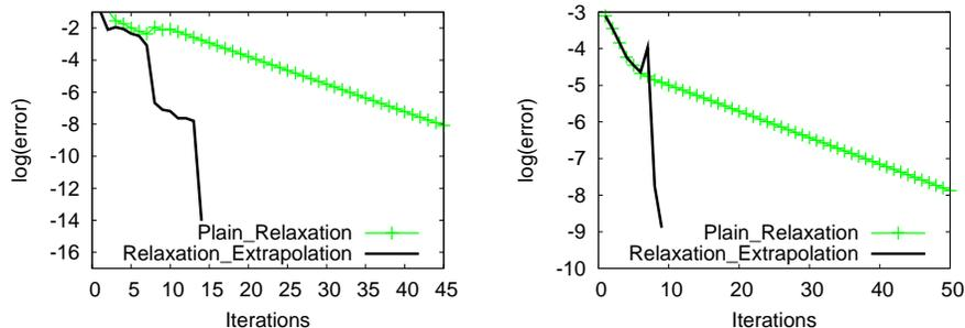
Figure 11: Comparison of errors for a single MESFET circuit and Colpitts Oscillator
