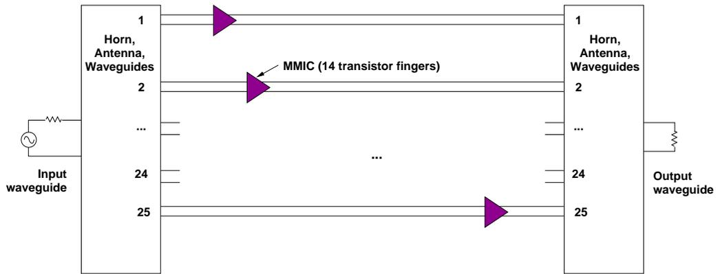
Figure 6: X-Band MMIC array spacial power combiner
