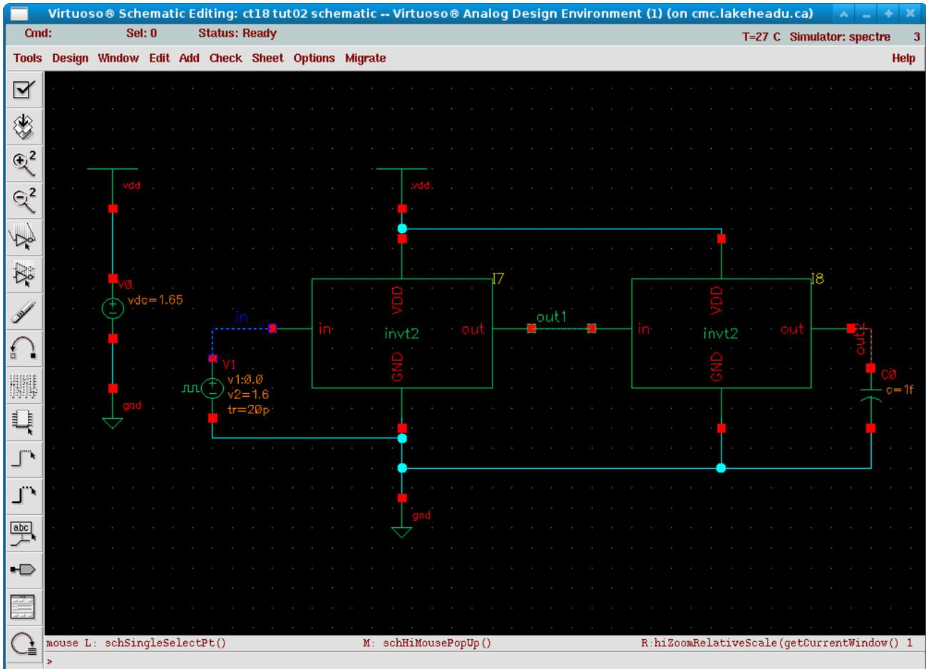
Next, create a new schematic in the same library that you are using to test the new symbol. The new created symbol can be instantiated as usual like other components, except that it located in is the Cell you are working with.
