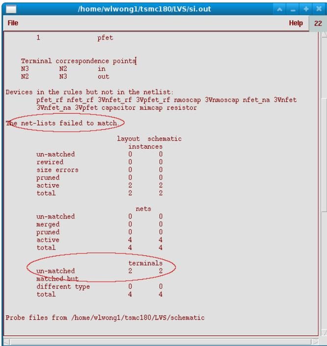
Click the **Output** button to display the report. Scroll down and look for the line “The net-lists failed to match” to verify there is no mismatch between the layout and schematic diagram. But if you follow the tutorial closely, you should find two errors in the report.
