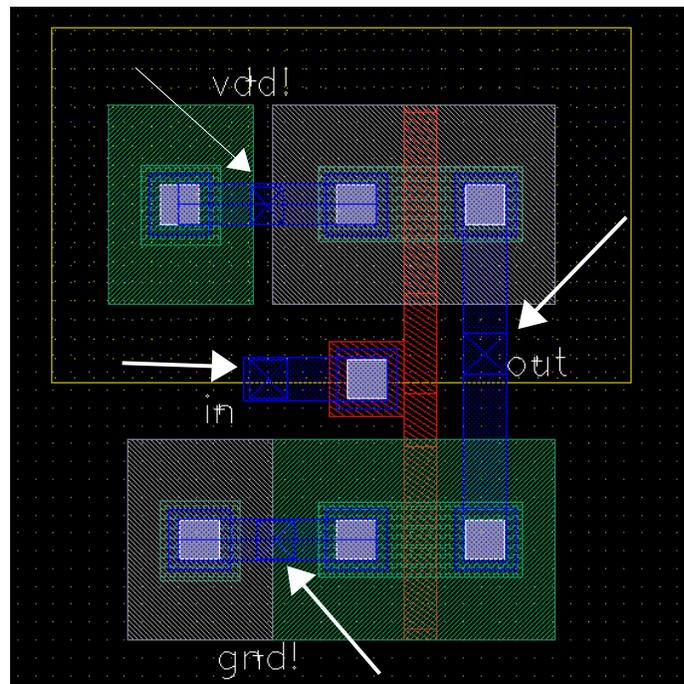
Fig. 10: Inverter Layout with Pins
