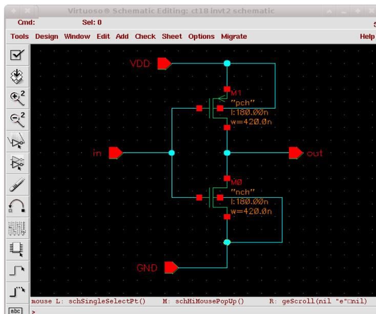
*Fig. 1: Schematic diagram. Change transistor width and length to 420 nm and 180 nm.*
